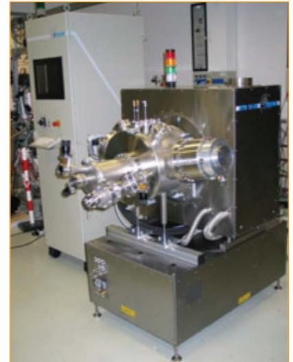
Figure 1. GDPP EUV source from Xtreme technologies. (Photo courtesy of Xtreme technologies).
