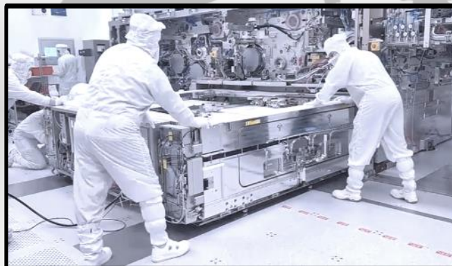
WAFER: Four main modules built, integration in progress, wafer stage motion under servo control
