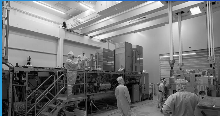
Forerunner POB installed in the system to de-risk new mechanics, actuator & electronics
