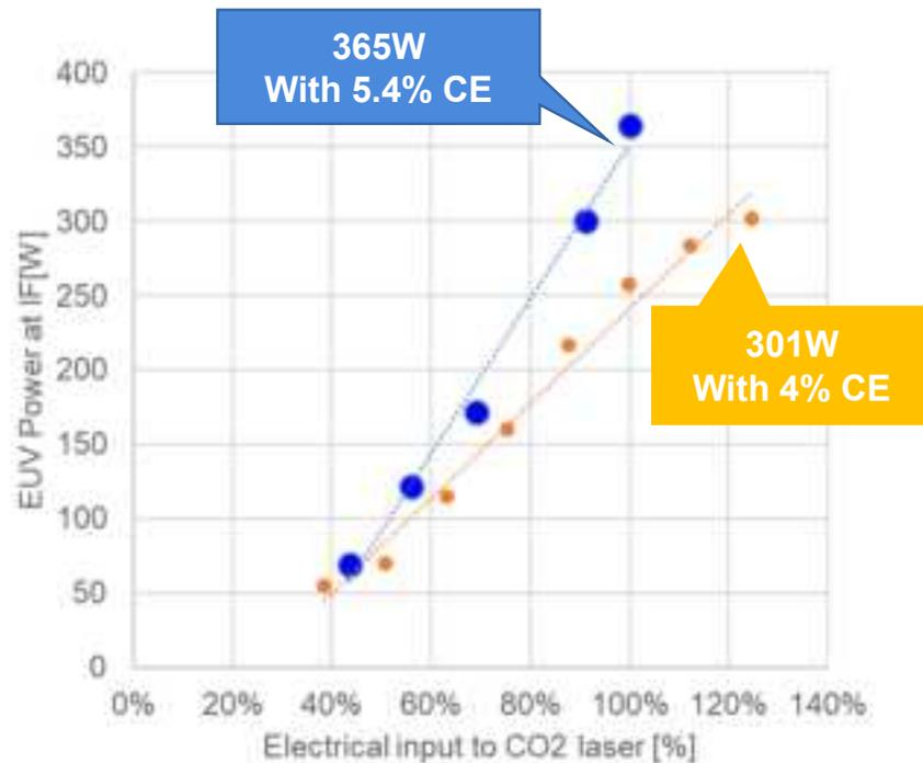
■ **Higher Droplet speed (>100m/s)** realized 1mm spacing and demonstrated more stable EUV generation
