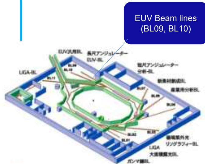
Two beam lines for EUV test in “New SUBARU”
