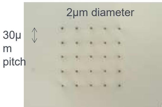
Hole diameter : 2μm
