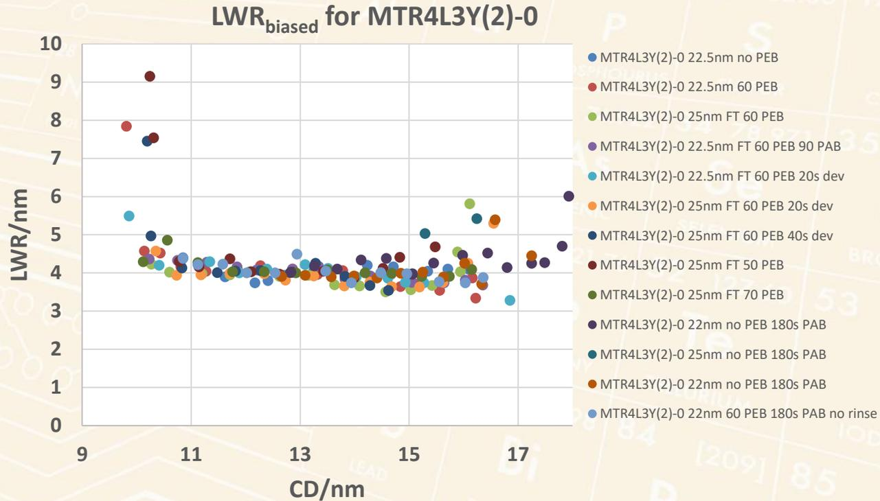
On the macro level, the LWR is remarkably level from 11nm to 15nm line width
