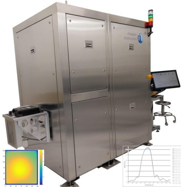
EUV mask blank reflectometer Inserts: AIMER Reflectivity map and reflectance curves over blank
