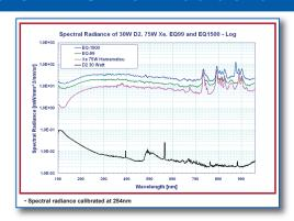
Near infrared diode laser beam is focused into a high pressure Xe bulb and a laser optical power sustained high temperature Xe plasma is generated. The plasma emits broad band radiation from 170nm to 1700nm with extremely high radiance (brightness).
