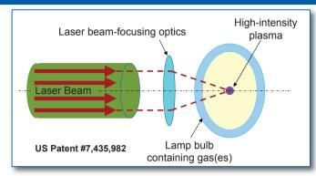
Near infrared diode laser beam is focused into a high pressure Xe bulb and a laser optical power sustained high temperature Xe plasma is generated. The plasma emits broad band radiation from 170nm to 1700nm with extremely high radiance (brightness).
