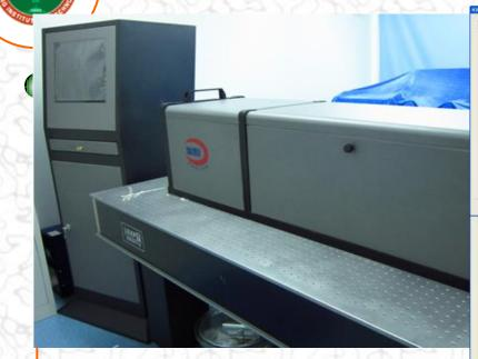
Absolute measurement accuracy: 5 nm rms. Measurement repeatability: 0.55 nm rms. Measurement Speed:20s/field point.
