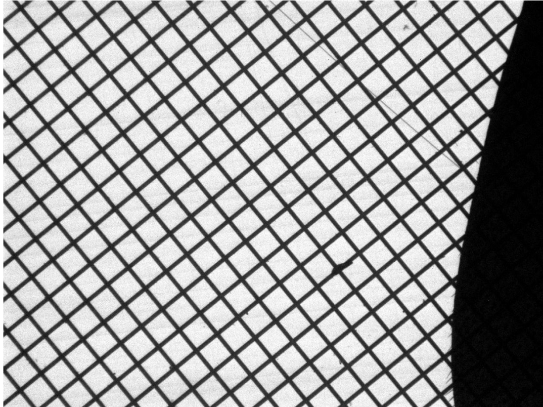
Fly wing on Ni mesh, 5 \mu\text{m} bars, 0.65 \mu\text{m} pixel size
