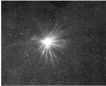
X-ray image of the laser plasma by the 17 mm EH microscope (IPPLM Warsaw)
