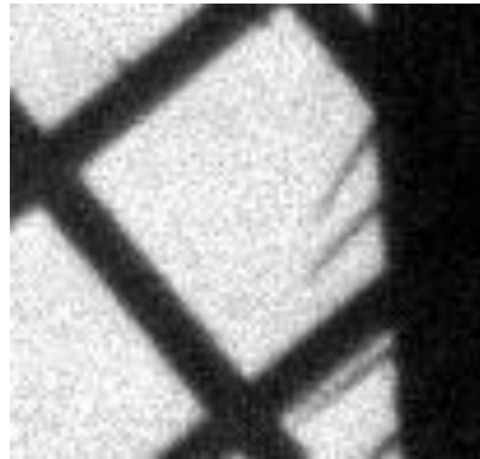
Fly wing on Ni mesh, 5 \mu\text{m} bars, 0.65 \mu\text{m} pixel size
