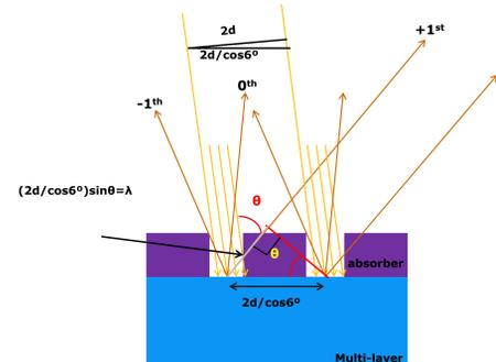
Fig. 5. The diffraction at EUV Mask
