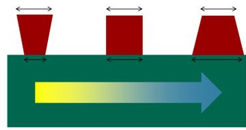
Fig. 4. ML area change with sidewall angle
