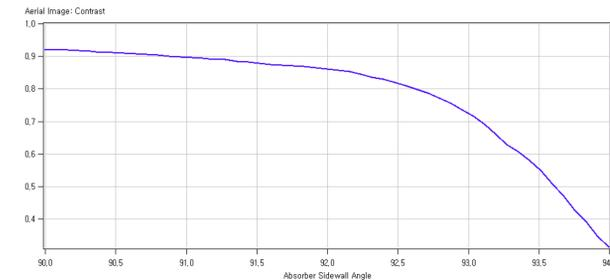
Fig. 3. Aerial image contrast degradation with sidewall angle variance
