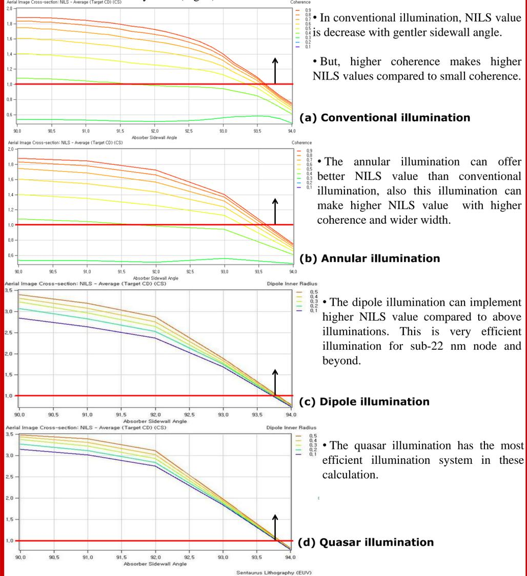
Fig. 9. Illumination parameters changes to eliminate the shadow effect
