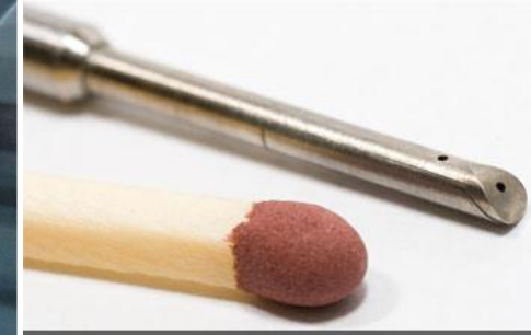
Figure 1:2 Sensor FRAP Probe with 1.8mm tip outer diameter of LEC.
