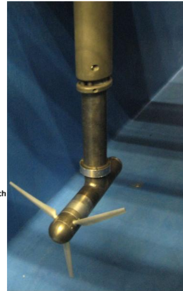
Figure 1:2 Sensor FRAP Probe with 1.8mm tip outer diameter of LEC.
