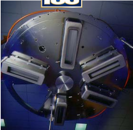
Underneath view of LLNL chamber lid with 5 sputtering targets
