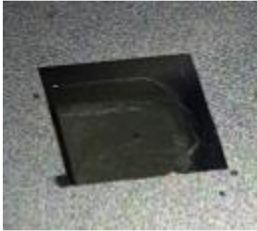
a-Si/graphene/a-Si membrane (100nm)
